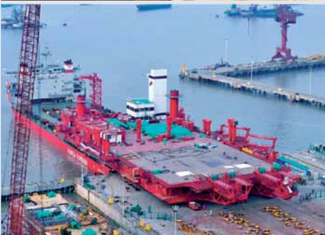
Roll-on operation for the 5,400-tonne upper hull block to be loaded onto the barge for delivery to Keppel FELS
