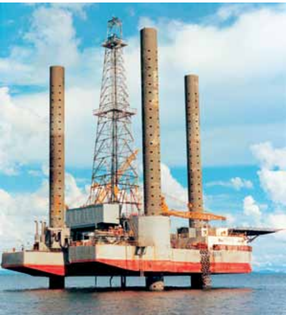
Keppel FELS has come a long way since it delivered its first jackup rig, JW Mclean in 1970
