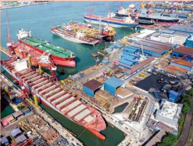
Keppel Shipyard achieved significant energy savings by installing regenerative energy systems in the yard cranes
