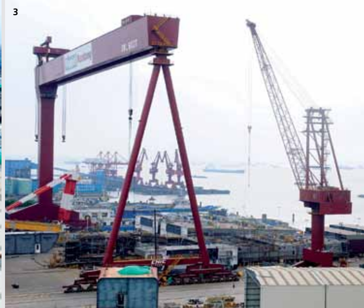
1. Keppel Nantong Shipyard and Keppel Nantong Heavy Industry – or collectively known as Keppel Nantong – have a total yard space of 43 hectares and are capable of taking on the construction work of a wide range of vessels and offshore structures; 2. Keppel Nantong's quayside is equipped with a 140-metre long slipway; 3. A 600-tonne gantry crane is part of the newly installed facilities in Keppel Nantong
