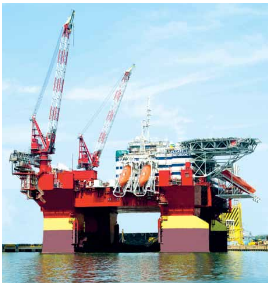
Floatel Endurance is built to Keppel's innovative DSS™ 20NS design which is able to work in the North Sea while at the same time remaining a cost-effective support semi wherever it is deployed
